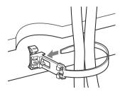
4 Tighten the cable tie by pulling its end.
